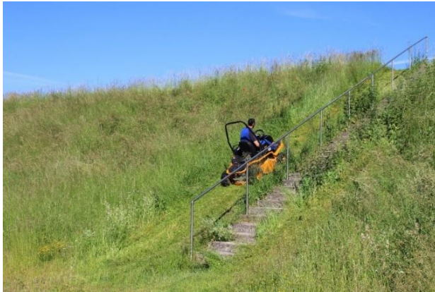
Photo 2: "When mowing the dams, we have to pay attention to the right time. If it is too wet, damage occurs that we drag along for years," explains dam keeper Martin Schmid.
