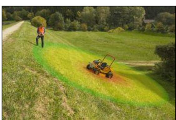
**Photo 1:** When the distance assistant is activated, the maximum driving speed, starting at a distance of approx. six metres to a distance of approx. two metres is gradually reduced to zero km/h
